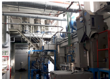
Picture 1, 2 and 3: The Romcolor's mega-compounder for whites and fillers uses silos for the polymers feeding (left). The line is equipped with state of the art upstream and downstream equipment (middle) and its packaging is supported by an industrial robot (right).
