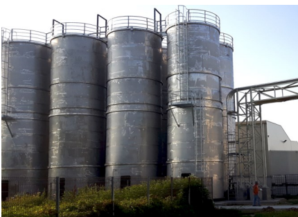
Picture 1, 2 and 3: The Romcolor's mega-compounder for whites and fillers uses silos for the polymers feeding (left). The line is equipped with state of the art upstream and downstream equipment (middle) and its packaging is supported by an industrial robot (right).
